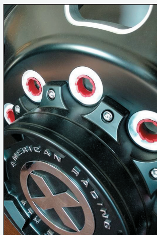
The Counteract Wheel Centering Sleeves in use.
